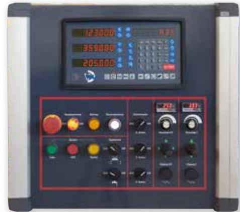
Tidy panel with standard 3-axis digital display and serial feed ads for X / Y- and Z-axis.
