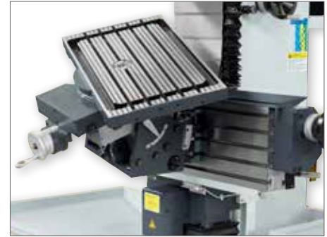
Universal rotaty-swivel table with 5 T-slots (14 H7, distance 63 mm) and 140 kg max. table load. (Option)
