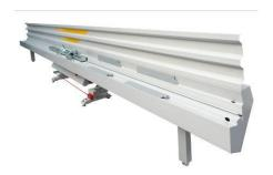
RAS technology and engineering have taken the seaming process from the traditional three steps, down to only one. In the past you had three different working steps: rollforming the receiver lock, rollforming or braking the flange and then closing the seam. The DuctZipper does it all in one smooth and simple operation!
